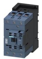
power contactor, AC-3e/AC-3, 95 A, 45 kW / 400 V, 3-pole, 24 V DC, 0.8-1.2\* Us, with integrated varistor, auxiliary contacts: 1 NO + 1 NC, integrated varistor, main circuit: screw terminal, control and auxiliary circuit: spring-loaded terminal, size: S3, suitable for PLC outputs
