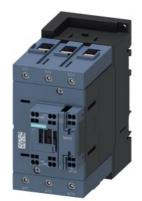
power contactor, AC-3e/AC-3, 95 A, 45 kW / 400 V, 3-pole, 400 V AC, 50 Hz / 400-440 V, 60 Hz, auxiliary contacts: 1 NO + 1 NC, main circuit: screw terminal, control and auxiliary circuit: spring-loaded terminal, size: S3
