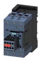
power contactor, AC-3e/AC-3, 95 A, 45 kW / 400 V, 3-pole, 24 V DC, 0.8-1.2\* Us, with integrated varistor, auxiliary contacts: 1 NO + 1 NC, screw terminal, size: S3, suitable for PLC outputs, captive auxiliary switch
