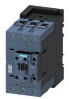
power contactor, AC-3e/AC-3, 95 A, 45 kW / 400 V, 3-pole, 24 V DC, 0.8-1.2\* Us, with integrated varistor, auxiliary contacts: 1 NO + 1 NC, screw terminal, size: S3, suitable for PLC outputs, upright mounting position
