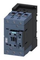
power contactor, AC-3e/AC-3, 95 A, 45 kW / 400 V, 3-pole, 400 V AC, 50 Hz, auxiliary contacts: 1 NO + 1 NC, screw terminal, size: S3  $\,$
