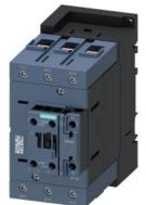
power contactor, AC-3e/AC-3, 95 A, 45 kW / 400 V, 3-pole, 500 V AC, 50/60 Hz, auxiliary contacts: 1 NO + 1 NC, screw terminal, size: S3  $\,$
