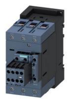
power contactor, AC-3e/AC-3, 95 A, 45 kW / 400 V, 3-pole, 230 V AC, 50 Hz, auxiliary contacts: 2 NO + 2 NC, screw terminal, size: S3, removable auxiliary switch
