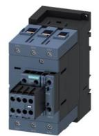
power contactor, AC-3e/AC-3, 95 A, 45 kW / 400 V, 3-pole, 220 V AC, 50/60 Hz, auxiliary contacts: 2 NO + 2 NC, screw terminal, size: S3, removable auxiliary switch
