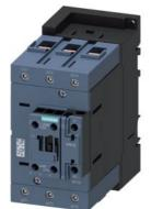
power contactor, AC-3e/AC-3, 95 A, 45 kW / 400 V, 3-pole, 125 V AC, 50 Hz, auxiliary contacts: 1 NO + 1 NC, screw terminal, size: S3
