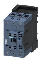
traction contactor, AC-3e/AC-3, 80 A, 37 kW / 400 V, 3-pole, 110 V DC, 0.7-1.25 $^{\star}$  Us, electronic drive, with integrated varistor, auxiliary contacts: 1 NO + 1 NC, main circuit: screw terminal, control and auxiliary circuit: spring-loaded terminal, size: S3
