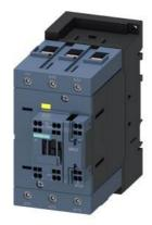
power contactor, AC-3e/AC-3, 80 A, 37 kW / 400 V, 3-pole, 21-33 V AC/DC, 50/60 Hz, with integrated varistor, auxiliary contacts: 1 NC, main circuit: screw terminal, control and auxiliary circuit: spring-loaded terminal, size: S3, F-PLC-IN
