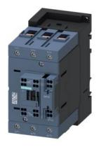
power contactor, AC-3e/AC-3, 80 A, 37 kW / 400 V, 3-pole, 24 V DC, 0.8-1.2\* Us, with integrated varistor, auxiliary contacts: 1 NO + 1 NC, integrated varistor, main circuit: screw terminal, control and auxiliary circuit: spring-loaded terminal, size: S3, suitable for PLC outputs
