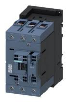
power contactor, AC-3e/AC-3, 80 A, 37 kW / 400 V, 3-pole, 400 V AC, 50 Hz, auxiliary contacts: 1 NO + 1 NC, main circuit: screw terminal, control and auxiliary circuit: spring-loaded terminal, size: S3  $\,$
