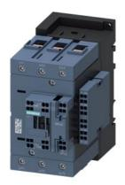
power contactor, AC-3e/AC-3, 80 A, 37 kW / 400 V, 3-pole, 230 V AC, 50 Hz, auxiliary contacts: 2 NO + 2 NC, main circuit: screw terminal, control and auxiliary circuit: spring-loaded terminal, size: S3, lateral auxiliary switch
