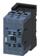
power contactor, AC-3e/AC-3, 80 A, 37 kW / 400 V, 3-pole, 208 V AC, 50/60 Hz, auxiliary contacts: 1 NO + 1 NC, main circuit: screw terminal, control and auxiliary circuit: spring-loaded terminal, size: S3
