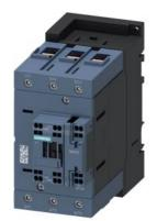
power contactor, AC-3e/AC-3, 80 A, 37 kW / 400 V, 3-pole, 110 V AC, 50 Hz / 120 V, 60 Hz, auxiliary contacts: 1 NO + 1 NC, main circuit: screw terminal, control and auxiliary circuit: spring-loaded terminal, size: S3
