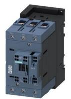
power contactor, AC-3e/AC-3, 80 A, 37 kW / 400 V, 3-pole, 110 V AC, 50/60 Hz, auxiliary contacts: 1 NO + 1 NC, main circuit: screw terminal, control and auxiliary circuit: spring-loaded terminal, size: S3
