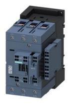
power contactor, AC-3e/AC-3, 80 A, 37 kW / 400 V, 3-pole, 110 V AC, 50 Hz, auxiliary contacts: 2 NO + 2 NC, main circuit: screw terminal, control and auxiliary circuit: spring-loaded terminal, size: S3, lateral auxiliary switch
