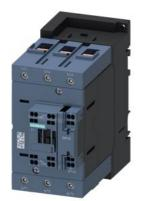
power contactor, AC-3e/AC-3, 80 A, 37 kW / 400 V, 3-pole, 24 V AC, 50/60 Hz, auxiliary contacts: 1 NO + 1 NC, main circuit: screw terminal, control and auxiliary circuit: spring-loaded terminal, size: S3
