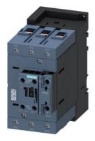
traction contactor, AC-3e/AC-3, 80 A, 37 kW / 400 V, 3-pole, 24 V DC, 0.7-1.25\* Us, electronic drive, with integrated varistor, auxiliary contacts: 1 NO + 1 NC, screw terminal, size: S3
