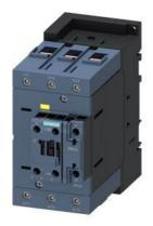
power contactor, AC-3e/AC-3, 80 A, 37 kW / 400 V, 3-pole, 83-150 V AC/DC, 50/60 Hz, with integrated varistor, auxiliary contacts: 1 NC, screw terminal, size: S3, F-PLC-IN
