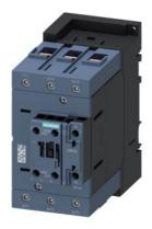
power contactor, AC-3e/AC-3, 80 A, 37 kW / 400 V, 3-pole, 83-155 V AC/DC, 50/60 Hz, with integrated varistor, auxiliary contacts: 1 NO + 1 NC, screw terminal, size: S3
