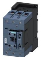
power contactor, AC-3e/AC-3, 80 A, 37 kW / 400 V, 3-pole, 48-80 V AC/DC, 50/60 Hz, with integrated varistor, auxiliary contacts: 1 NO + 1 NC, screw terminal, size: S3
