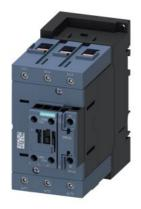
power contactor, AC-3e/AC-3, 80 A, 37 kW / 400 V, 3-pole, 20-33 V AC/DC, 50/60 Hz, with integrated varistor, auxiliary contacts: 1 NO + 1 NC, screw terminal, size: S3  $\,$
