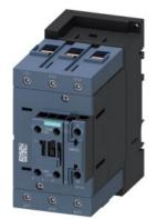
power contactor, AC-3e/AC-3, 80 A, 37 kW / 400 V, 3-pole, 24 V DC, 0.8-1.2\* Us, with integrated varistor, auxiliary contacts: 1 NO + 1 NC, screw terminal, size: S3, suitable for PLC outputs
