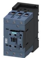
power contactor, AC-3e/AC-3, 80 A, 37 kW / 400 V, 3-pole, 24 V DC, 0.8-1.2\* Us, with integrated varistor, auxiliary contacts: 1 NO + 1 NC, screw terminal, size: S3, suitable for PLC outputs, upright mounting position
