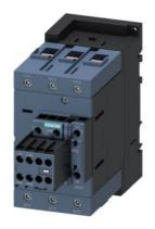
power contactor, AC-3e/AC-3, 80 A, 37 kW / 400 V, 3-pole, 230 V AC, 50 Hz, auxiliary contacts: 2 NO + 2 NC, screw terminal, size: S3, removable auxiliary switch
