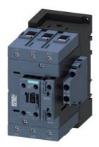
power contactor, AC-3e/AC-3, 80 A, 37 kW / 400 V, 3-pole, 230 V AC, 50/60 Hz, auxiliary contacts: 2 NO + 2 NC, screw terminal, size: S3, lateral auxiliary switch
