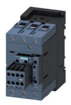
power contactor, AC-3e/AC-3, 80 A, 37 kW / 400 V, 3-pole, 230 V AC, 50/60 Hz, auxiliary contacts: 2 NO + 2 NC, screw terminal, size: S3, removable auxiliary switch
