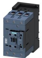
power contactor, AC-3e/AC-3, 80 A, 37 kW / 400 V, 3-pole, 110 V AC, 50 Hz / 120 V, 60 Hz, auxiliary contacts: 1 NO + 1 NC, screw terminal, size: S3  $\,$
