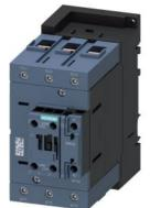
power contactor, AC-3e/AC-3, 80 A, 37 kW / 400 V, 3-pole, 24 V AC, 50/60 Hz, auxiliary contacts: 1 NO + 1 NC, screw terminal, size: S3  $\,$
