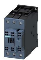
traction contactor, AC-3e/AC-3, 80 A, 37 kW / 400 V, 3-pole, 72 V DC, 0.7-1.25\* Us, electronic drive, with integrated varistor, auxiliary contacts: 1 NO + 1 NC, main circuit: screw terminal, control and auxiliary circuit: spring-loaded terminal, size: S2
