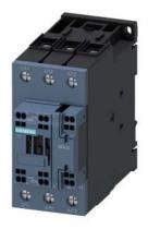
traction contactor, AC-3e/AC-3, 80 A, 37 kW / 400 V, 3-pole, 24 V DC, 0.7-1.25\* Us, electronic drive, with integrated varistor, auxiliary contacts: 1 NO + 1 NC, main circuit: screw terminal, control and auxiliary circuit: spring-loaded terminal, size: S2
