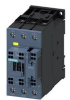
power contactor, AC-3e/AC-3, 80 A, 37 kW / 400 V, 3-pole, 83-150 V AC/DC, 50/60 Hz, with integrated varistor, auxiliary contacts: 1 NC, main circuit: screw terminal, control and auxiliary circuit: spring-loaded terminal, size: S2, F-PLC-IN
