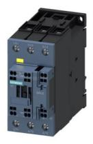
power contactor, AC-3e/AC-3, 80 A, 37 kW / 400 V, 3-pole, 21-33 V AC/DC, 50/60 Hz, with integrated varistor, auxiliary contacts: 1 NC, main circuit: screw terminal, control and auxiliary circuit: spring-loaded terminal, size: S2, F-PLC-IN
