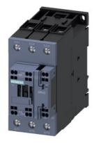
power contactor, AC-3e/AC-3, 80 A, 37 kW / 400 V, 3-pole, 175-280 V AC/DC, 50/60 Hz, with integrated varistor, auxiliary contacts: 1 NO + 1 NC, main circuit: screw terminal, control and auxiliary circuit: spring-loaded terminal, size: S2,
