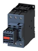
power contactor, AC-3e/AC-3, 80 A, 37 kW / 400 V, 3-pole, 24 V DC, 0.8-1.2\* Us, with integrated varistor, auxiliary contacts: 2 NO + 2 NC, main circuit: screw terminal, control and auxiliary circuit: spring-loaded terminal, size: S2, suitable for PLC outputs, captive auxiliary switch
