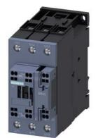
power contactor, AC-3e/AC-3, 80 A, 37 kW / 400 V, 3-pole, 208 V AC, 50/60 Hz, auxiliary contacts: 1 NO + 1 NC, main circuit: screw terminal, control and auxiliary circuit: spring-loaded terminal, size: S2
