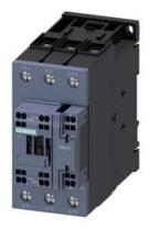
power contactor, AC-3e/AC-3, 80 A, 37 kW / 400 V, 3-pole, 230 V AC, 50/60 Hz, auxiliary contacts: 1 NO + 1 NC, main circuit: screw terminal, control and auxiliary circuit: spring-loaded terminal, size: S2
