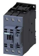
power contactor, AC-3e/AC-3, 80 A, 37 kW / 400 V, 3-pole, 110 V AC, 50/60 Hz, auxiliary contacts: 1 NO + 1 NC, main circuit: screw terminal, control and auxiliary circuit: spring-loaded terminal, size: S2
