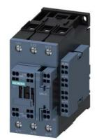
power contactor, AC-3e/AC-3, 80 A, 37 kW / 400 V, 3-pole, 110 V AC, 50 Hz, auxiliary contacts: 2 NO + 2 NC, main circuit: screw terminal, control and auxiliary circuit: spring-loaded terminal, size: S2, lateral auxiliary switch
