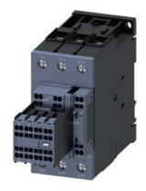
power contactor, AC-3e/AC-3, 80 A, 37 kW / 400 V, 3-pole, 110 V AC, 50 Hz, auxiliary contacts: 2 NO + 2 NC, main circuit: screw terminal, control and auxiliary circuit: spring-loaded terminal, size: S2, removable auxiliary switch
