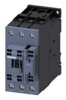
power contactor, AC-3e/AC-3, 80 A, 37 kW / 400 V, 3-pole, 110 V AC, 50 Hz, auxiliary contacts: 1 NO + 1 NC, main circuit: screw terminal, control and auxiliary circuit: spring-loaded terminal, size: S2
