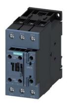
traction contactor, AC-3e/AC-3, 80 A, 37 kW / 400 V, 3-pole, 110 V DC, 0.7-1.25\* Us, electronic drive, with integrated varistor, auxiliary contacts: 1 NO + 1 NC, screw terminal, size: S2
