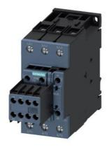
power contactor, AC-3e/AC-3, 80 A, 37 kW / 400 V, 3-pole, 175-280 V AC/DC, 50/60 Hz, with integrated varistor, auxiliary contacts: 2 NO + 2 NC, screw terminal, size: S2, removable auxiliary switch
