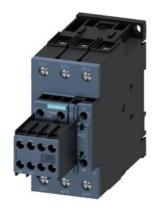
power contactor, AC-3e/AC-3, 80 A, 37 kW / 400 V, 3-pole, 24 V DC, 0.8-1.2\* Us, with integrated varistor, auxiliary contacts: 2 NO + 2 NC, screw terminal, size: S2, suitable for PLC outputs, removable auxiliary switch
