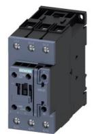
power contactor, AC-3e/AC-3, 80 A, 37 kW / 400 V, 3-pole, 24 V DC, 0.8-1.2\* Us, with integrated varistor, auxiliary contacts: 1 NO + 1 NC, screw terminal, size: S2, suitable for PLC outputs
