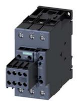
power contactor, AC-3e/AC-3, 80 A, 37 kW / 400 V, 3-pole, 400 V AC, 50 Hz, auxiliary contacts: 2 NO + 2 NC, screw terminal, size: S2, removable auxiliary switch
