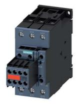
power contactor, AC-3e/AC-3, 80 A, 37 kW / 400 V, 3-pole, 230 V AC, 50 Hz, auxiliary contacts: 2 NO + 2 NC, screw terminal, size: S2, captive auxiliary switch
