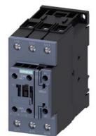
power contactor, AC-3e/AC-3, 80 A, 37 kW / 400 V, 3-pole, 230 V AC, 50 Hz, auxiliary contacts: 1 NO + 1 NC, screw terminal, size: S2  $\,$
